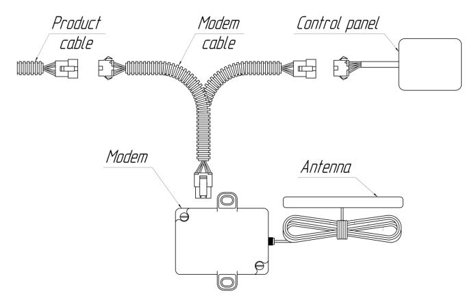
Fig. 3. Modem connection to AUTOTERM heaters
